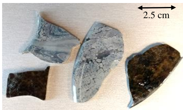
Figure 2. Optical image of the as-received glass. The darker side is the side of the melt that was in contact with the Inconel plate when the melt was quenched.
