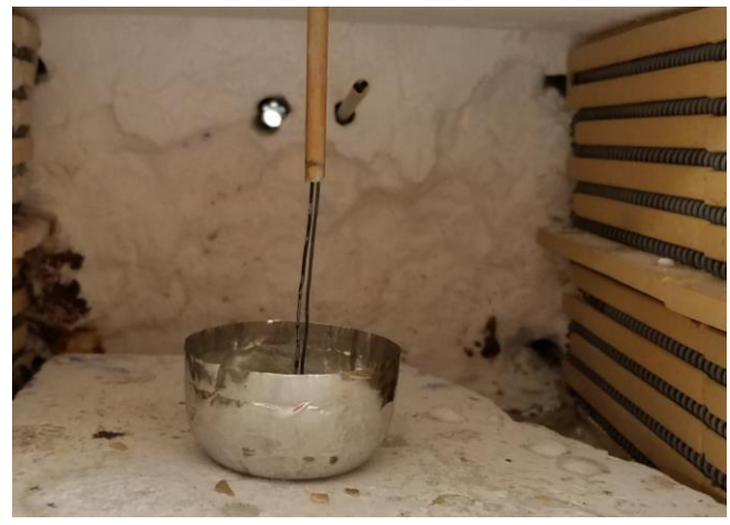
Figure 5. Furnace cool experiment with embedded thermocouple.
